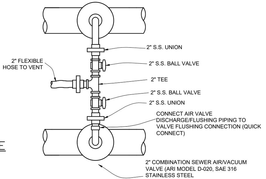
PLAN – AIR VALVE INSTALLATION
