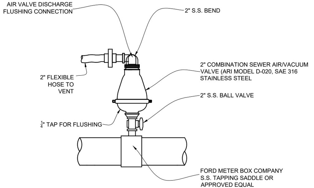
SECTION – AIR VALVE INSTALLATION
