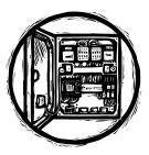
**DO** locate your electrical control panel where it will be protected from potential vandalism and have unobstructed access.
