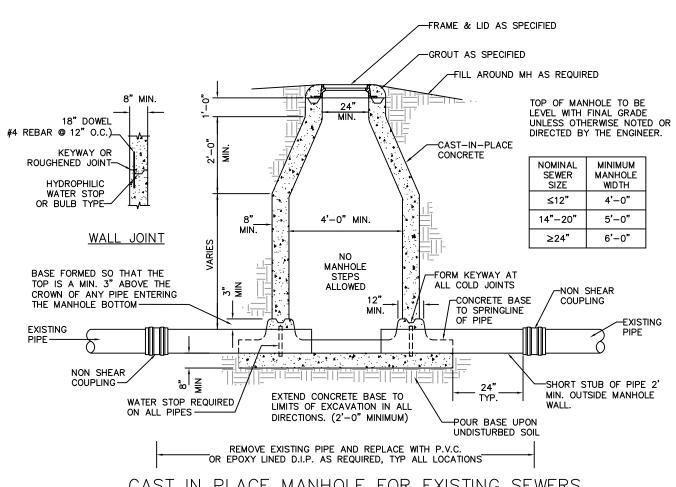
CAST IN PLACE MANHOLE FOR EXISTING SEWERS
