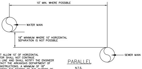
IF CONDITIONS WILL NOT ALLOW 10' OF HORIZONTAL SEPARATION, CONTRACTOR SHALL NOT CONTINUE CONSTRUCTION OF THIS LINE AND SHALL NOTIFY THE ENGINEER SO THAT HE MAY CONTACT THE ARKANSAS DEPARTMENT OF HEALTH FOR FURTHER INSTRUCTIONS. A MINIMUM OF 18" SHALL BE MAINTAINED FROM THE BOTTOM OF THE OUTSIDE OF WATER MAIN TO THE CROWN OF THE SEWER AND THE WATER MAIN SHALL BE DUCTILE IRON.
